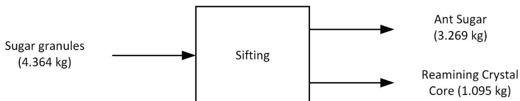
Figure 8. Mass balance in the sieving process at the level of crystal coconut sugar craftsmen
