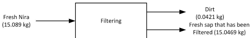
Figure 3. Mass balance at the sugar craftsman level filtering process crystal coconut
