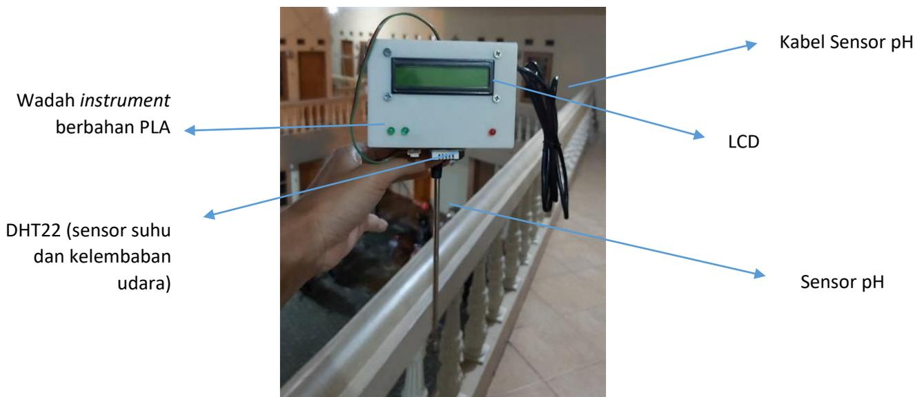
Gambar 5. Alat Monitoring Otomatis berbasis Web
